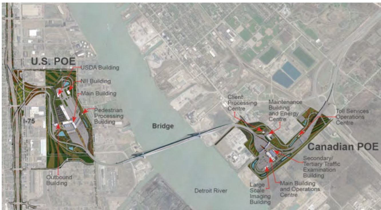
Figure 1: Components of the Gordie Howe International Bridge
